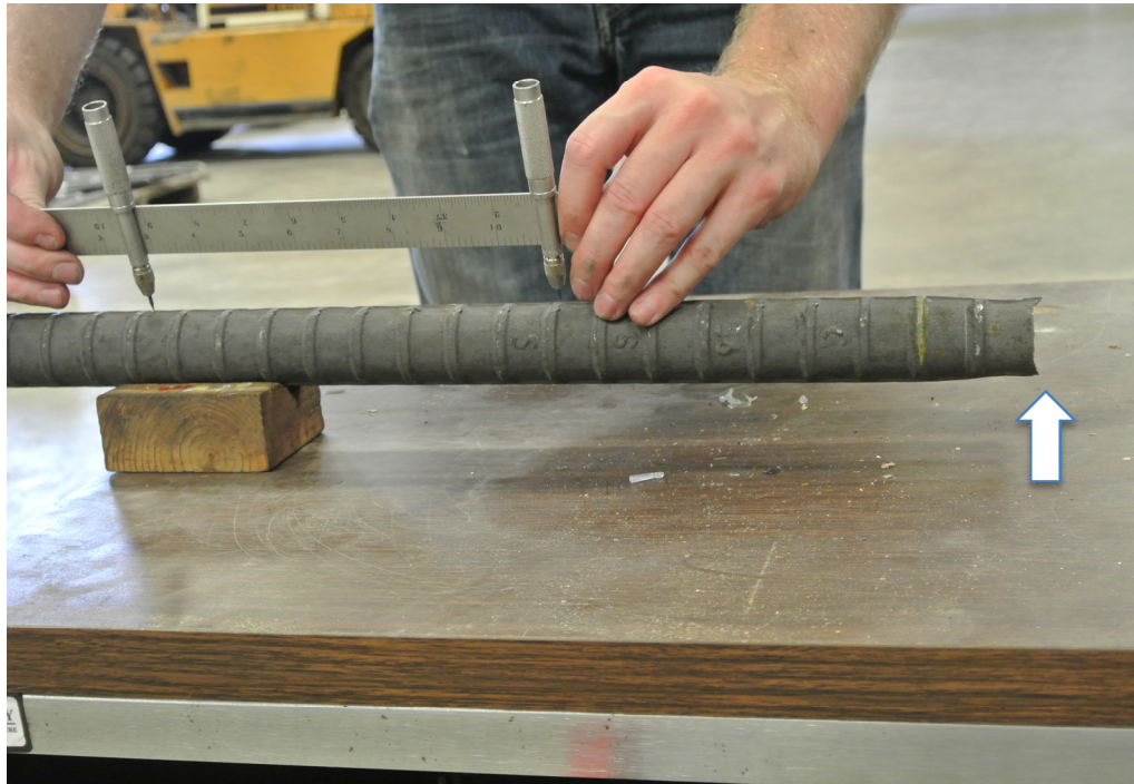
Figure 2-3 Photo of uniform elongation being measured. Arrow points to fracture location (photo courtesy of Wiss, Janney, Elstner Associates, Inc., Copyright 2013).
